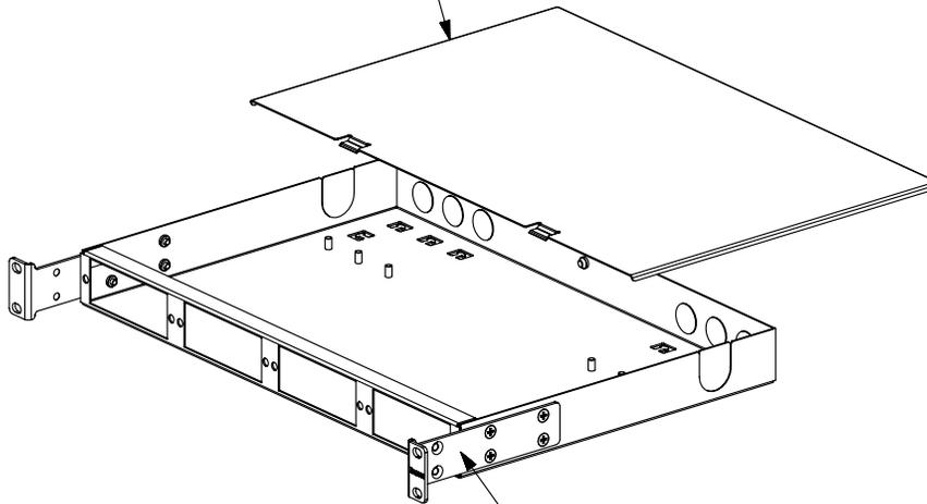
ENCLOSURE MOUNTING BRACKET (INSTALLED)
