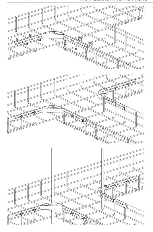
Assemble (1) radius support bracket to baskets. Keep supplied fasteners loose.
